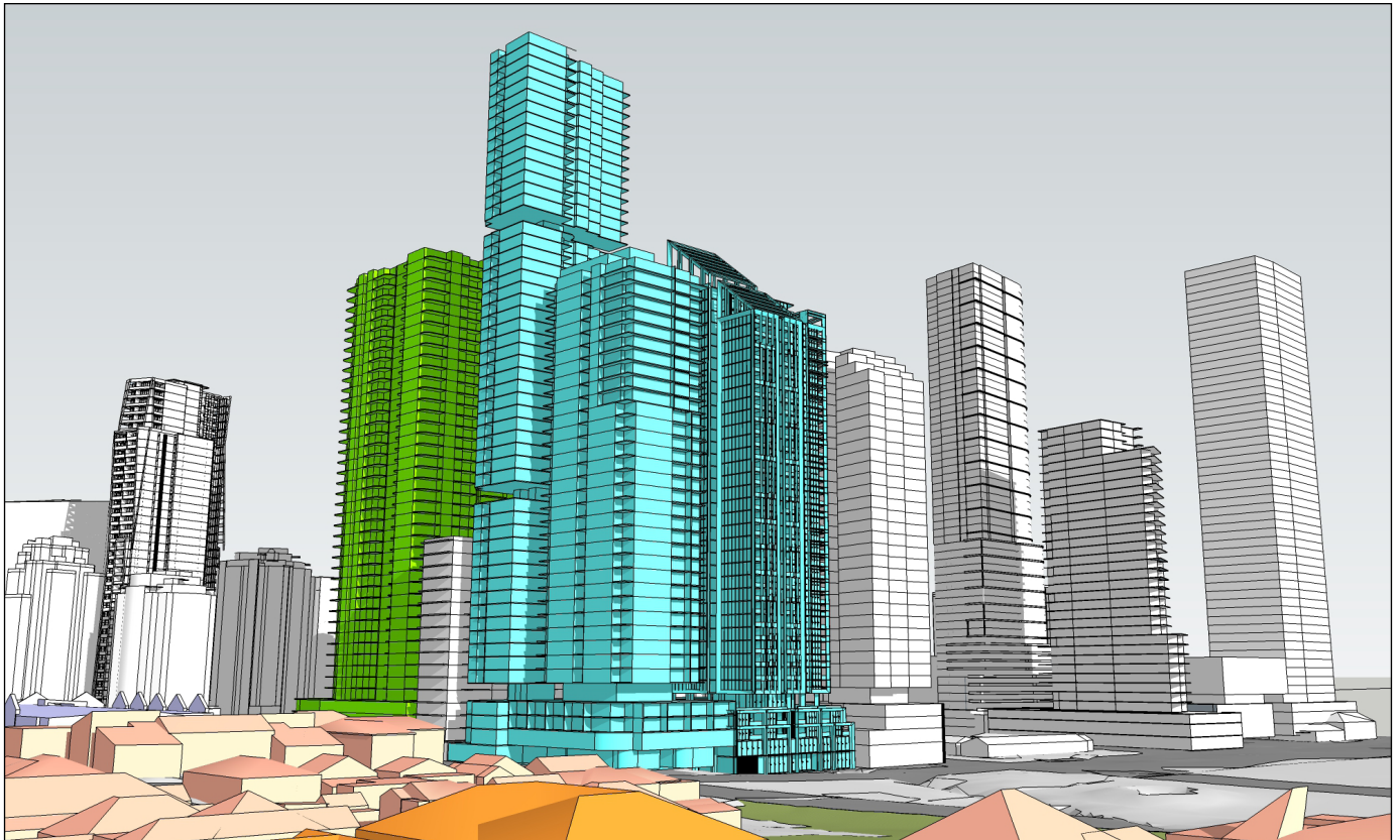
Massing study for proposed developments as supplied to CLA. Used for solar access analysis.
